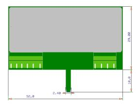
The Transponder module is equipped with two connectors, for connection to the amplifier main board
